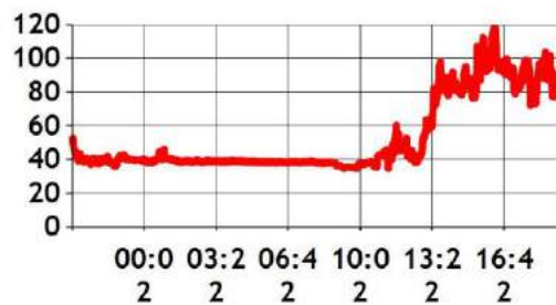
RMS CURRENT VARIATION TIME PLOT OF CH3
